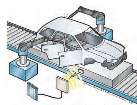
▲ A basic RFID system consists of a tag on the item being tracked, an antenna to transmit and receive the data communication to and from the tag, and the computer system to which it is linked. Widely used in automotive assembly and production applications, RFID systems like the one shown here can function as a set of plans and specifications that travels with the workpiece. For example, the system might both tell a robotic station what operation to perform and record what has been accomplished.
